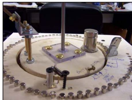
FIGURE 10. Photo of 6” rotor in the potential energy well at end of cycle.
